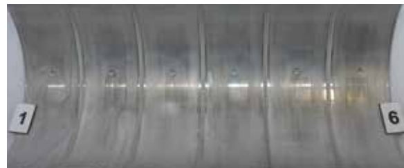
Bearings after 200,000 km of service with TRACTION PRO LS 5W30 - MAN testing area
